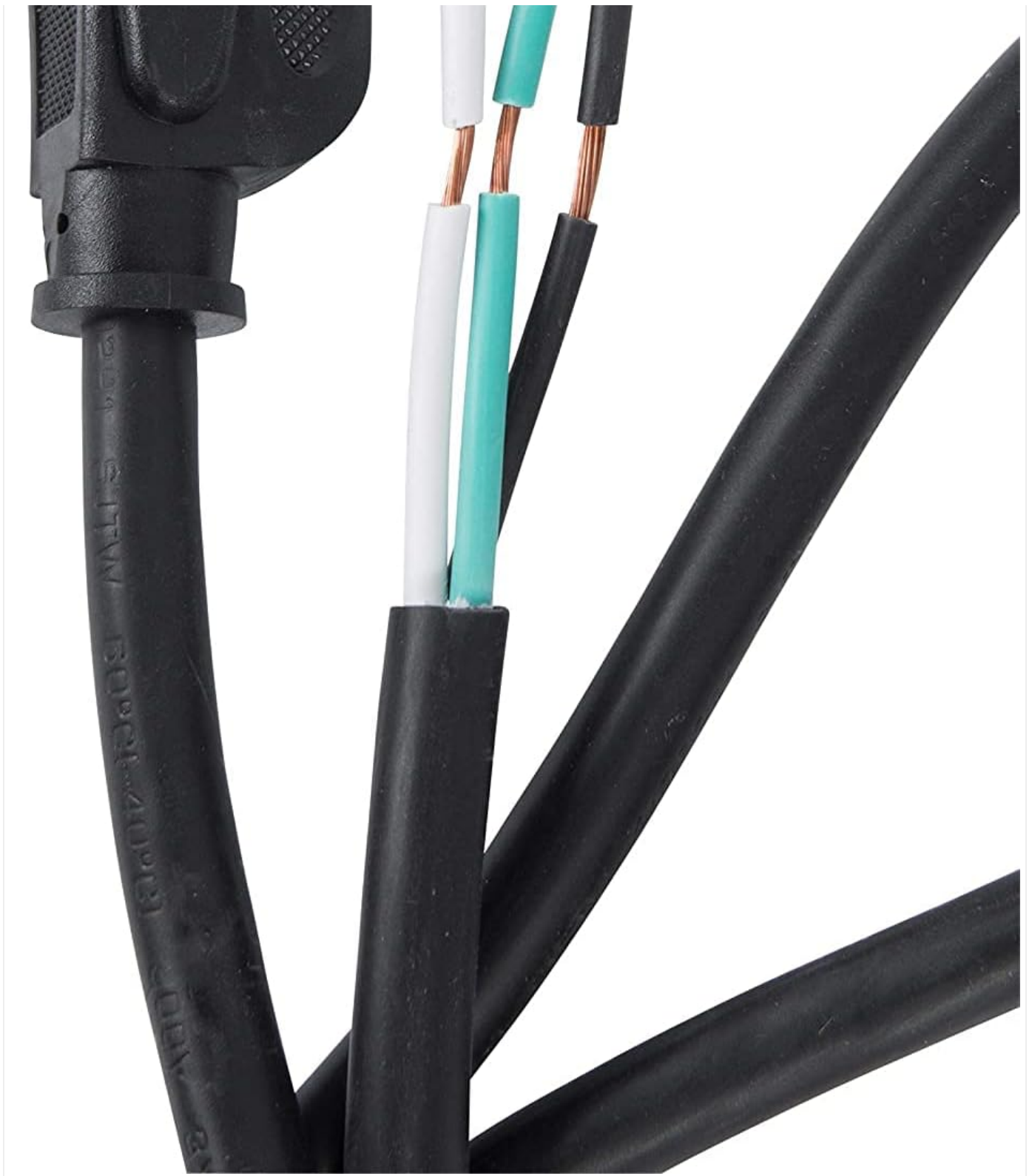
Image: A detailed view of the bare wire ends of the power cord, showing the white (neutral), green (ground), and black (live) insulated conductors ready for connection.
