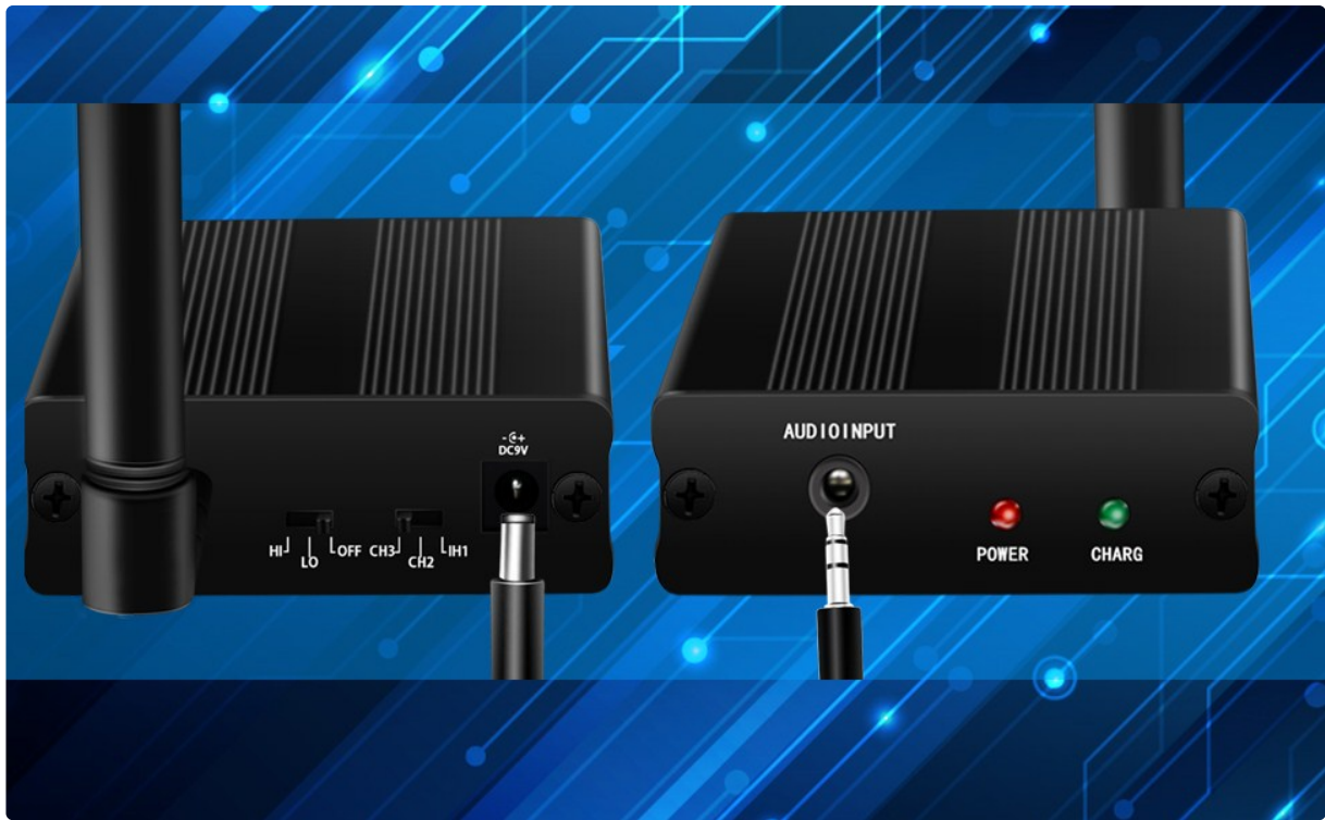
Figure 4: The UHF transmitter unit with its connection ports.
