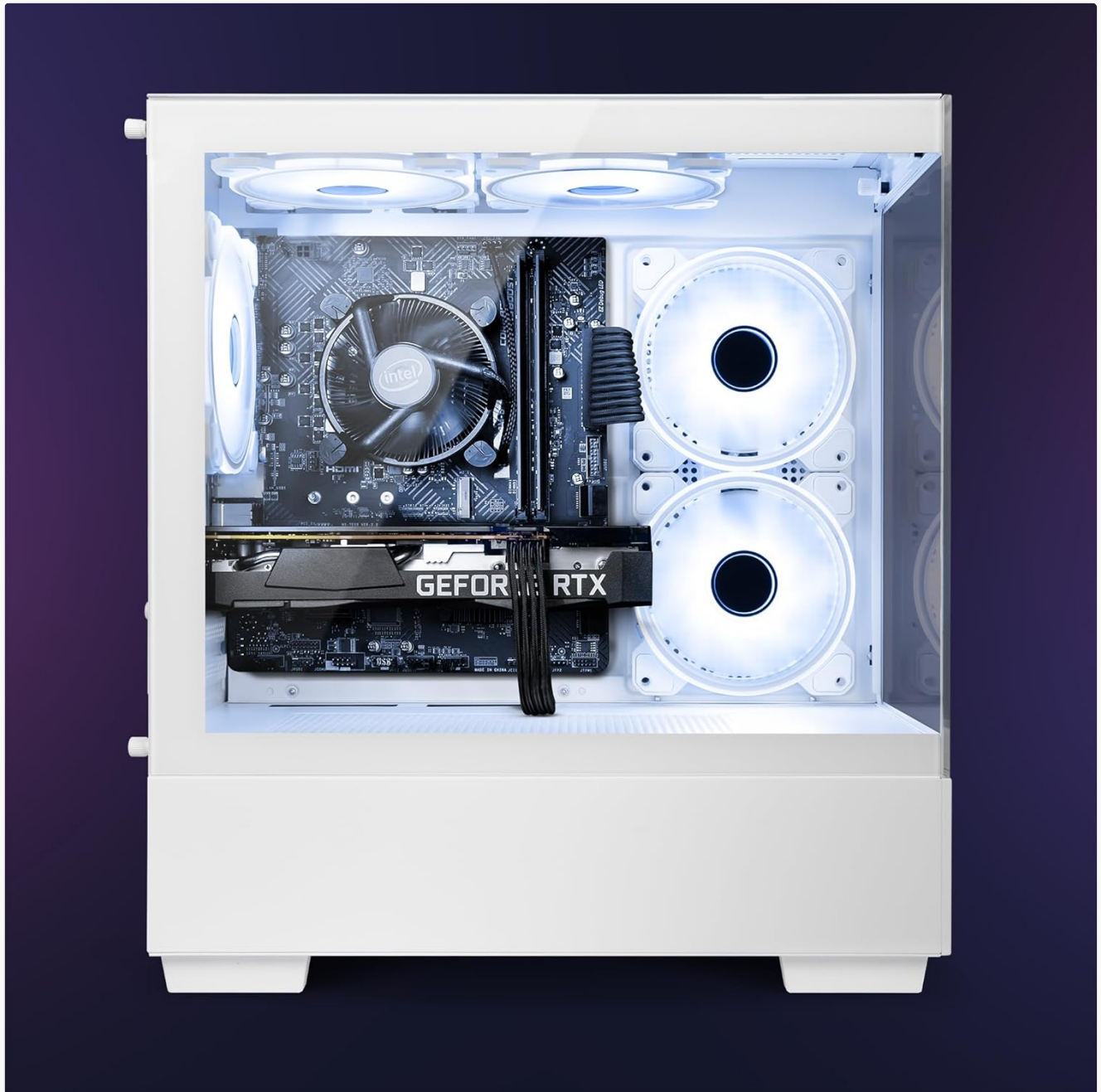
Image 2.1: Internal view of the PC, highlighting the Intel CPU cooler and the Nvidia GeForce RTX 3060 graphics card.
