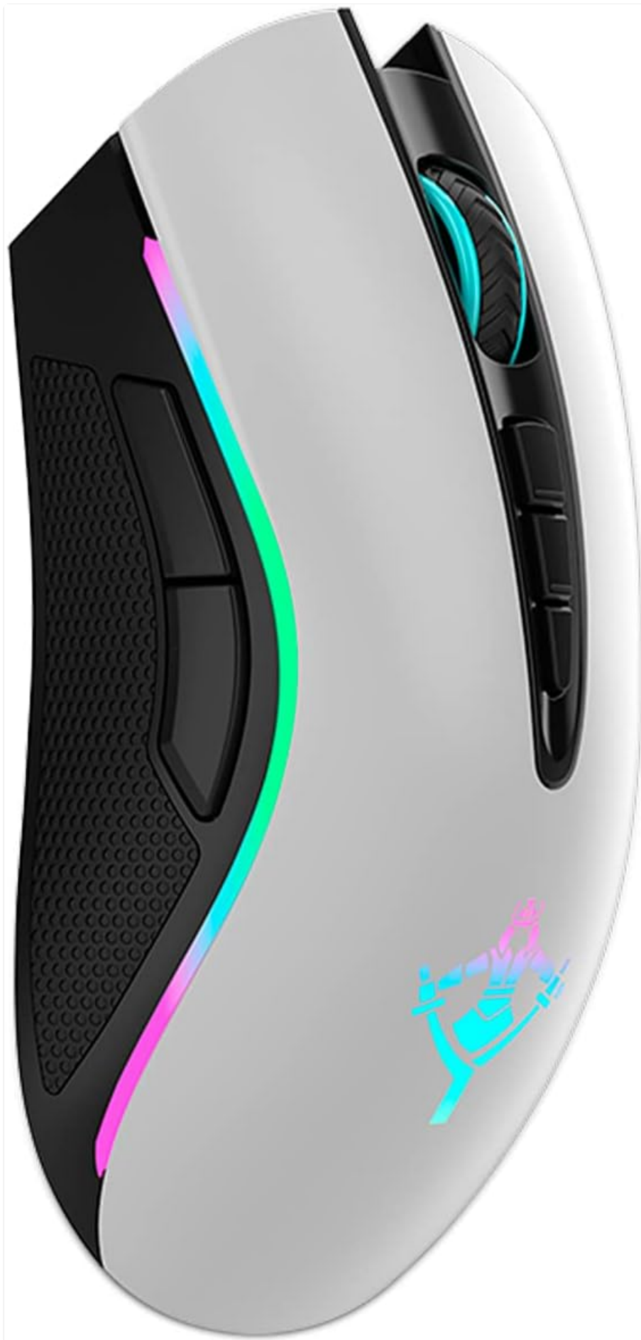
Figure 4: An angled view of the mouse, illustrating the placement of the scroll wheel and side buttons, which are key for DPI adjustment and programmable functions.
