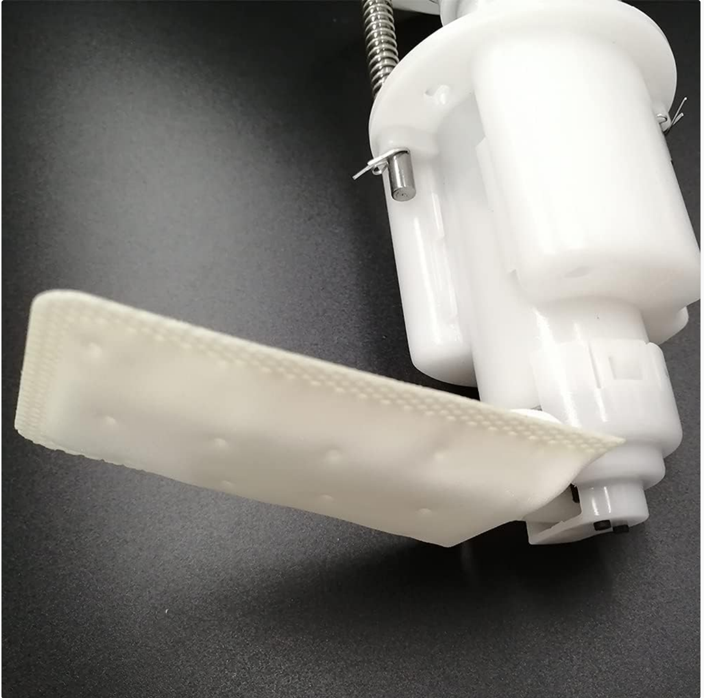
Image: The fuel filter or strainer, an integral part of the fuel pump assembly, designed to prevent debris from entering the pump and fuel system.
