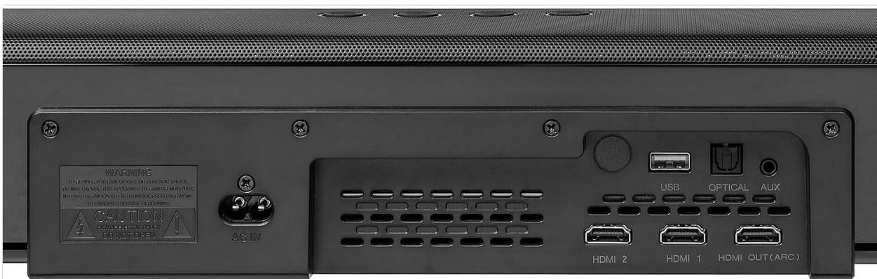
The rear panel of the sound bar features various input and output ports for connecting to external devices. These include HDMI 1, HDMI 2, HDMI OUT (ARC), Optical, USB, and AUX inputs, along with the AC power input.
