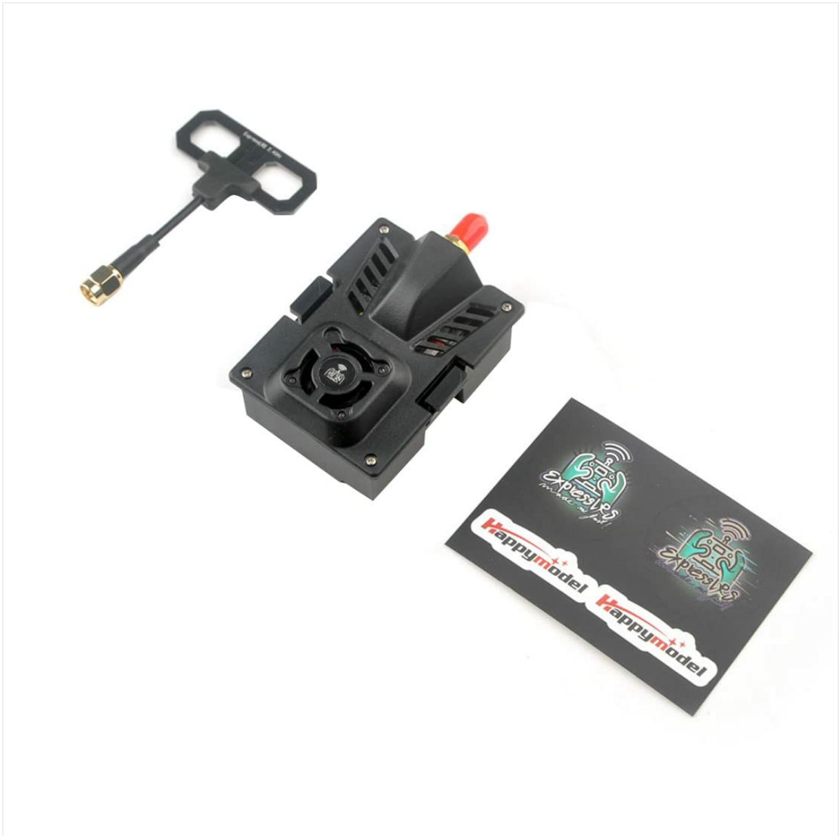
Figure 4.1: Front view of the ES24TX Pro module with the Moxon antenna attached.
