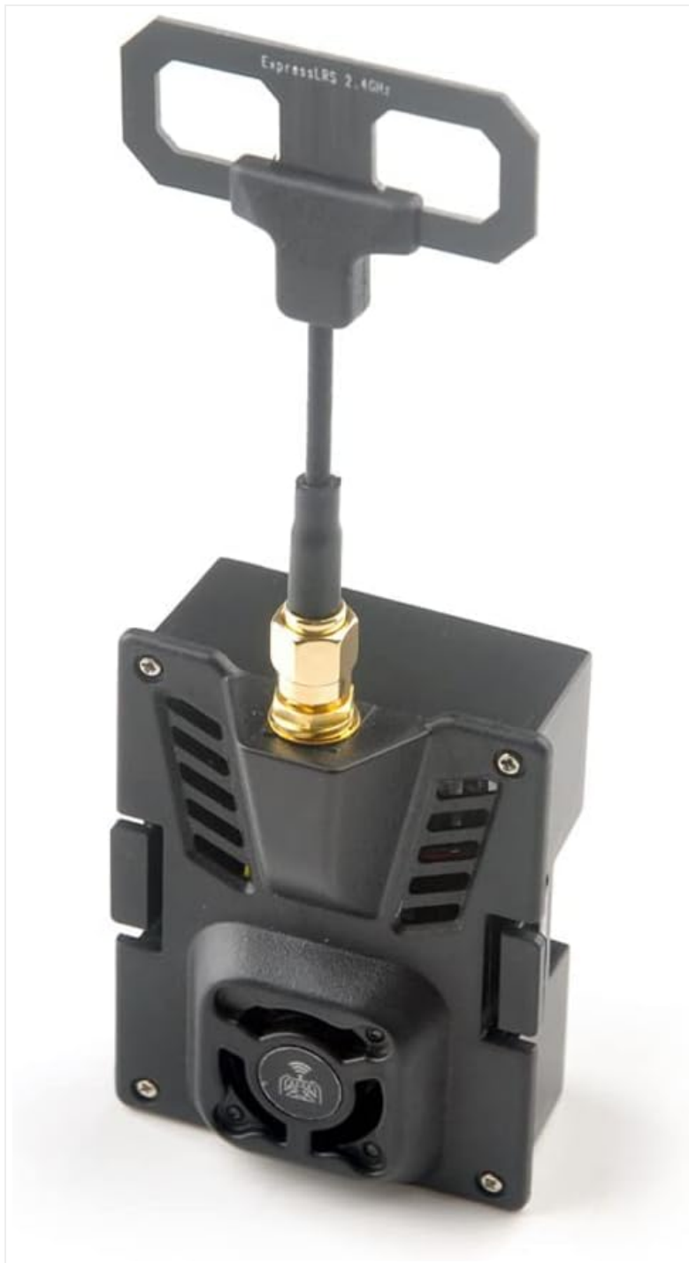
Figure 4.2: The ES24TX Pro module and its included Moxon antenna.
