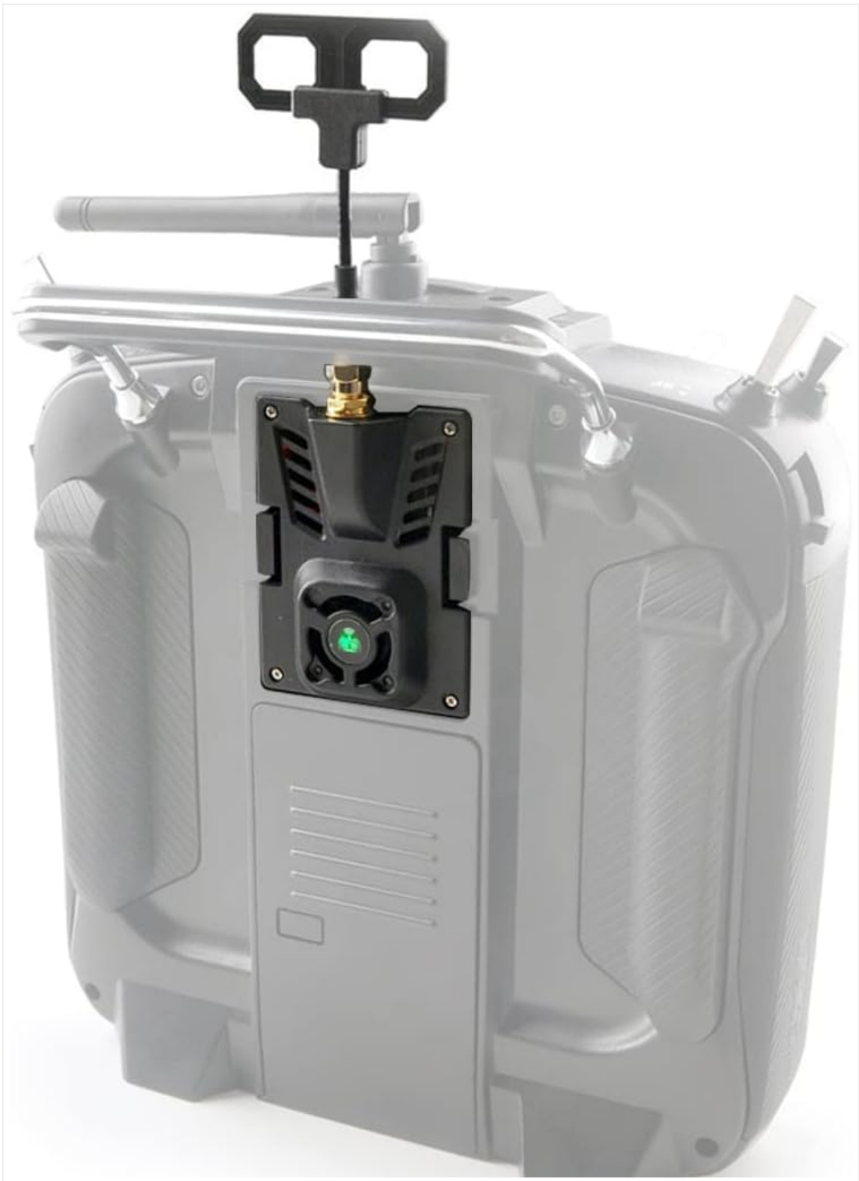
Figure 5.3: Close-up of the module's fan and RGB LED when installed on a radio transmitter.
