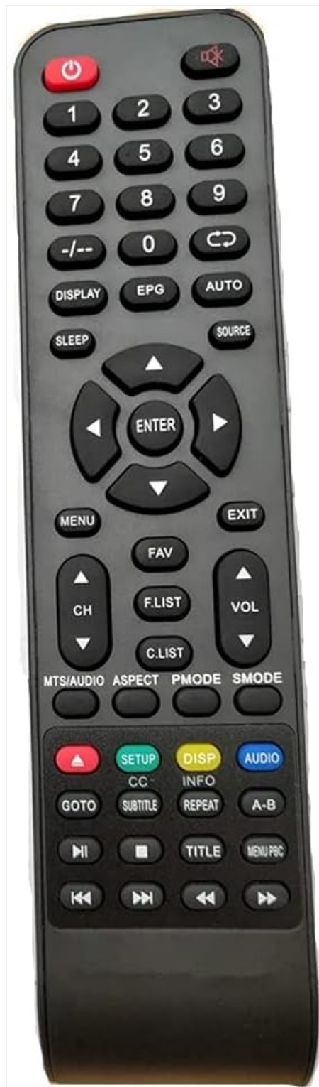
Image 1: Front view of the Bestol remote control, showing all buttons including power, number pad, navigation, volume, channel, and media controls.
