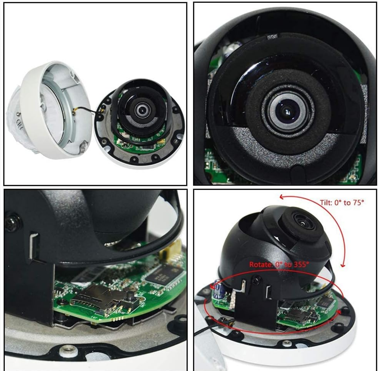
Image: Disassembled view of the camera showing internal components and adjustable lens for rotation and tilt. This illustrates the camera's internal structure and adjustability.
