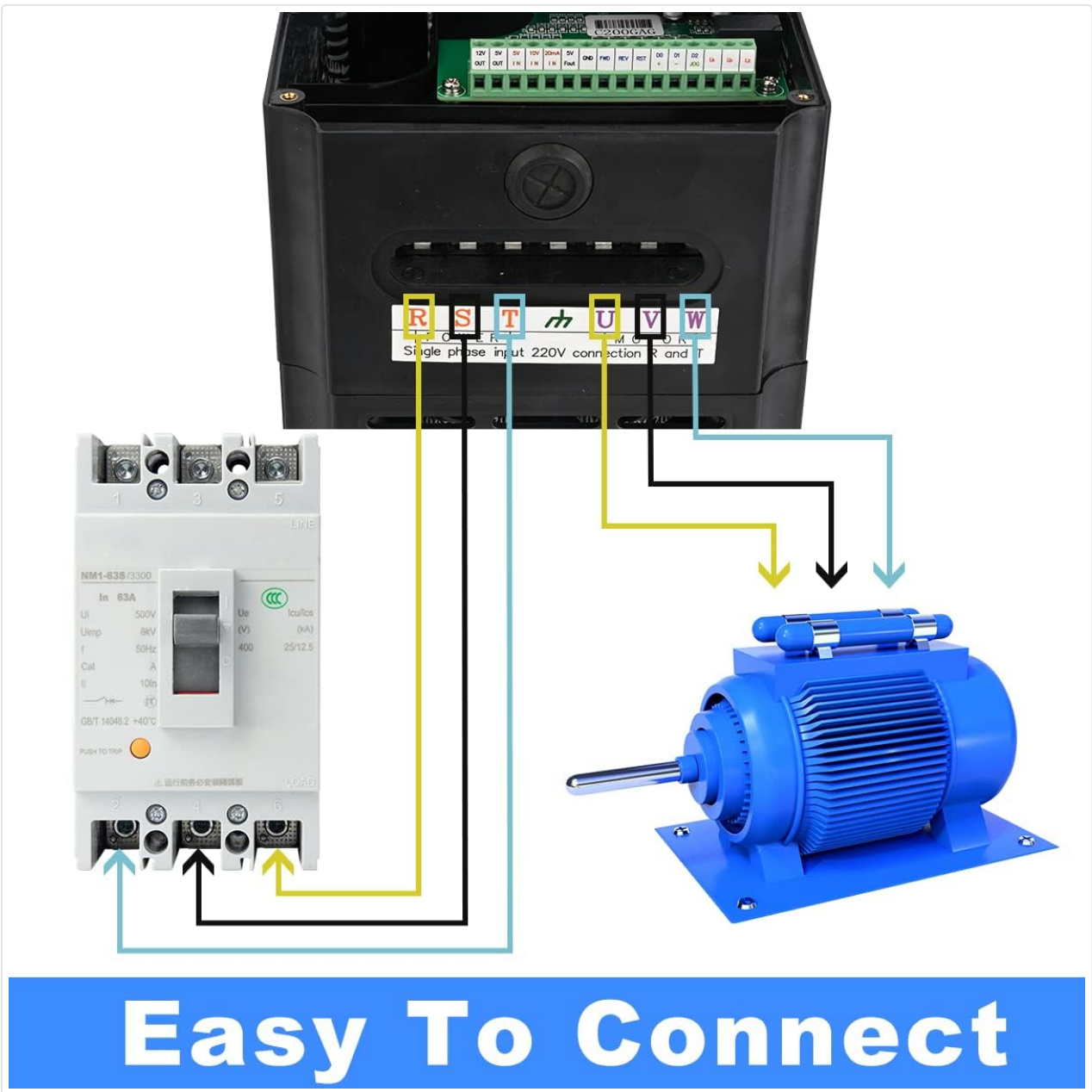
Figure 2: Simplified power connection diagram for the VFD.
