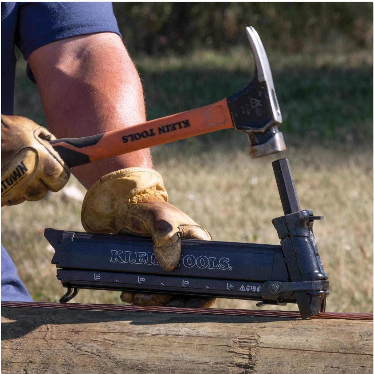
Image 3.1: A user demonstrating the proper technique of striking the staple starter with a hammer to secure a staple.
