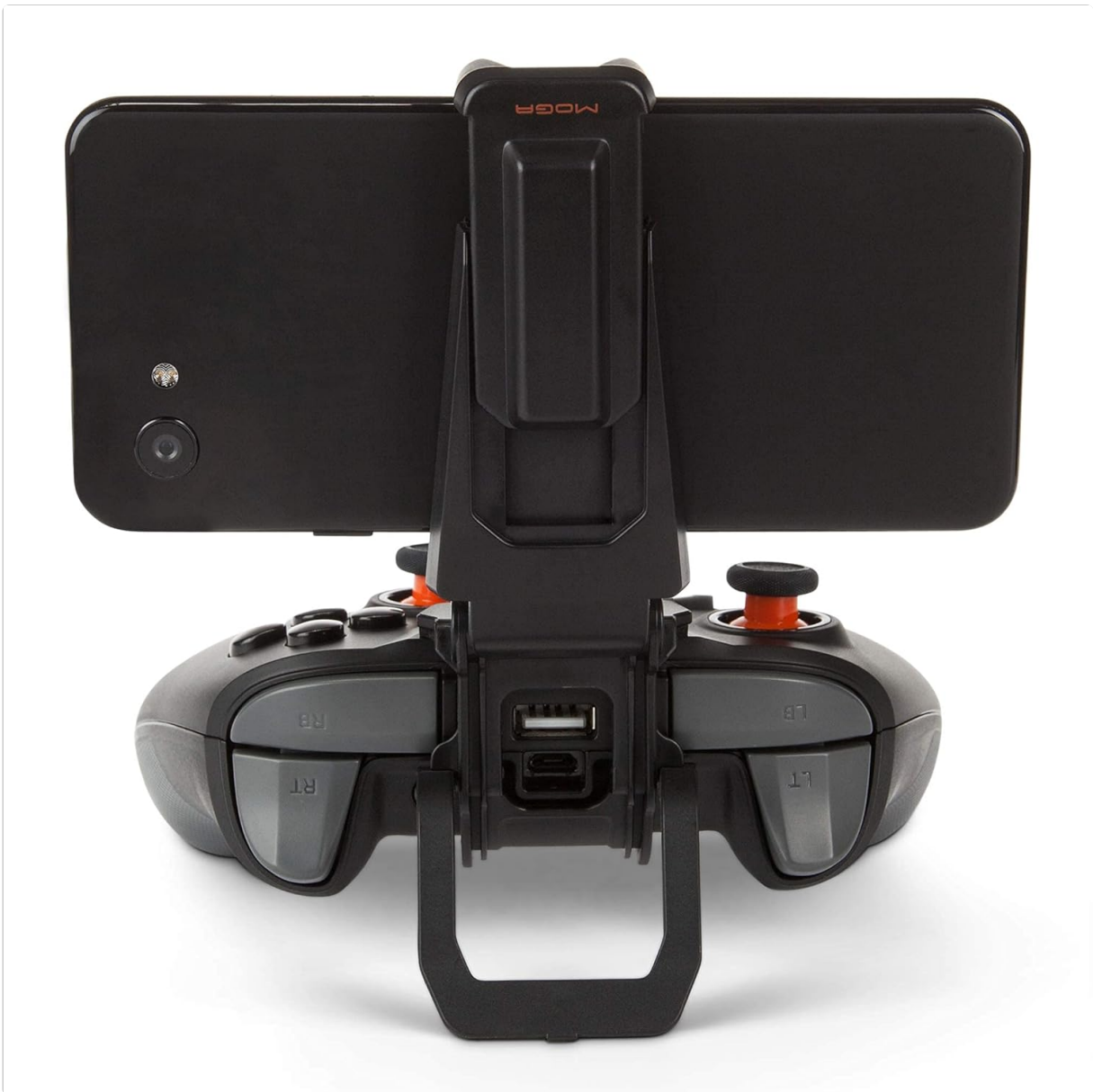
Image: Rear view of the PowerA MOGA XP5-A Plus controller with the phone clip extended. The image highlights the USB-C port for controller charging and the USB-A port for charging a mobile device.
