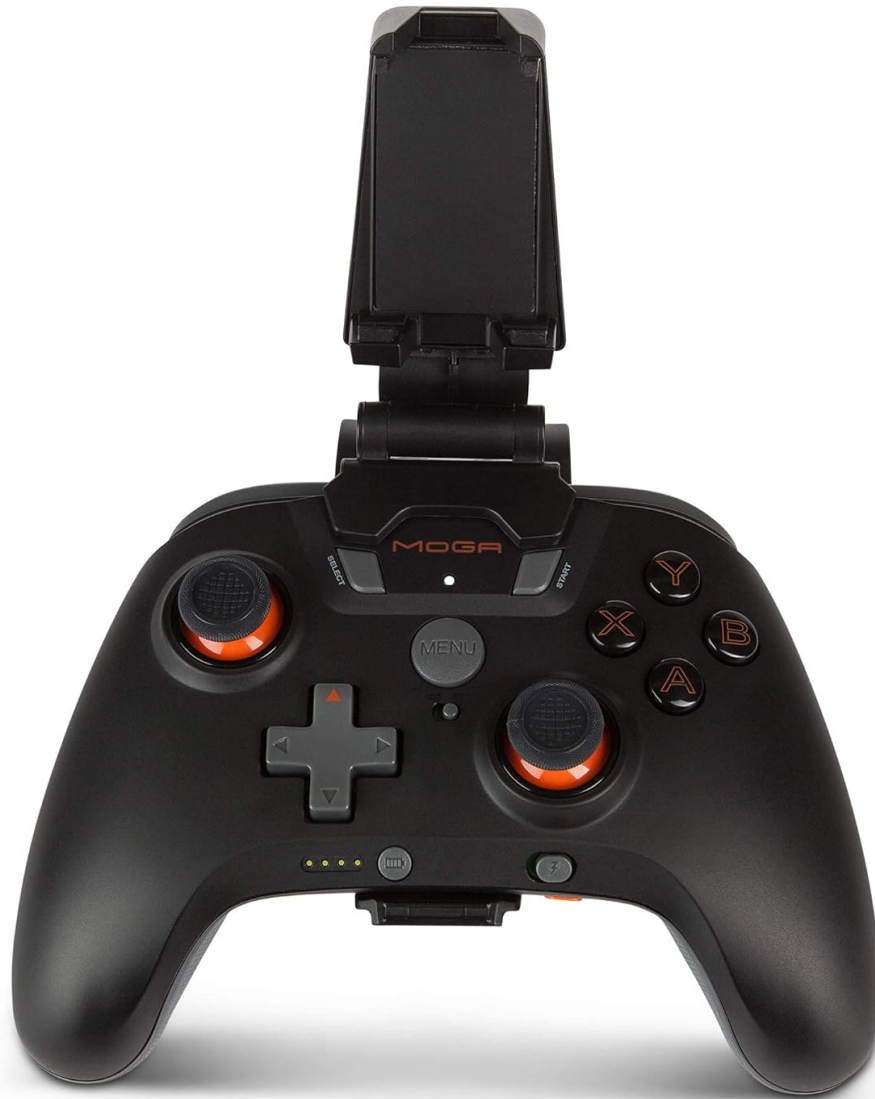
Image: Top-down view of the PowerA MOGA XP5-A Plus controller. The phone clip is folded back, showing the dual analog sticks, D-pad, ABXY buttons, Menu, Select, Start buttons, and LED indicators.
