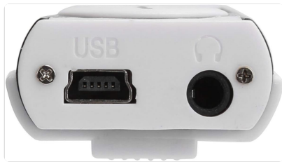
Figure 2: Bottom view showing the USB charging/data port and headphone jack.
