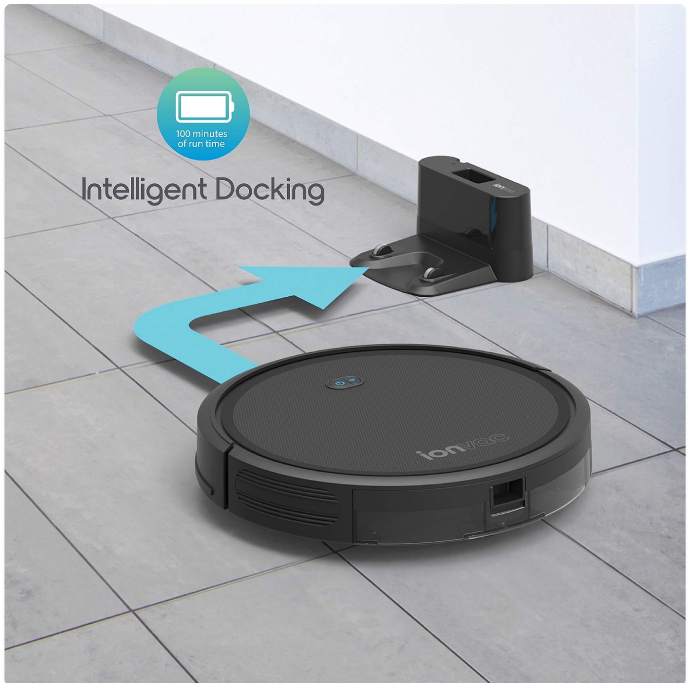
Figure 4.1: The Robovac demonstrating its intelligent docking capability, returning to its charging station automatically after cleaning or when battery is low.
