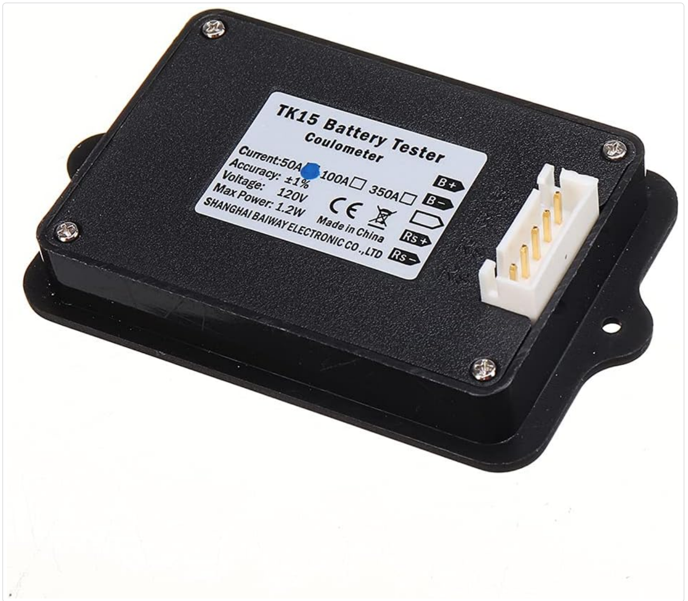
Figure 3.1: Rear view of the TK15 Coulomb Meter, showing the model number and current rating information.
