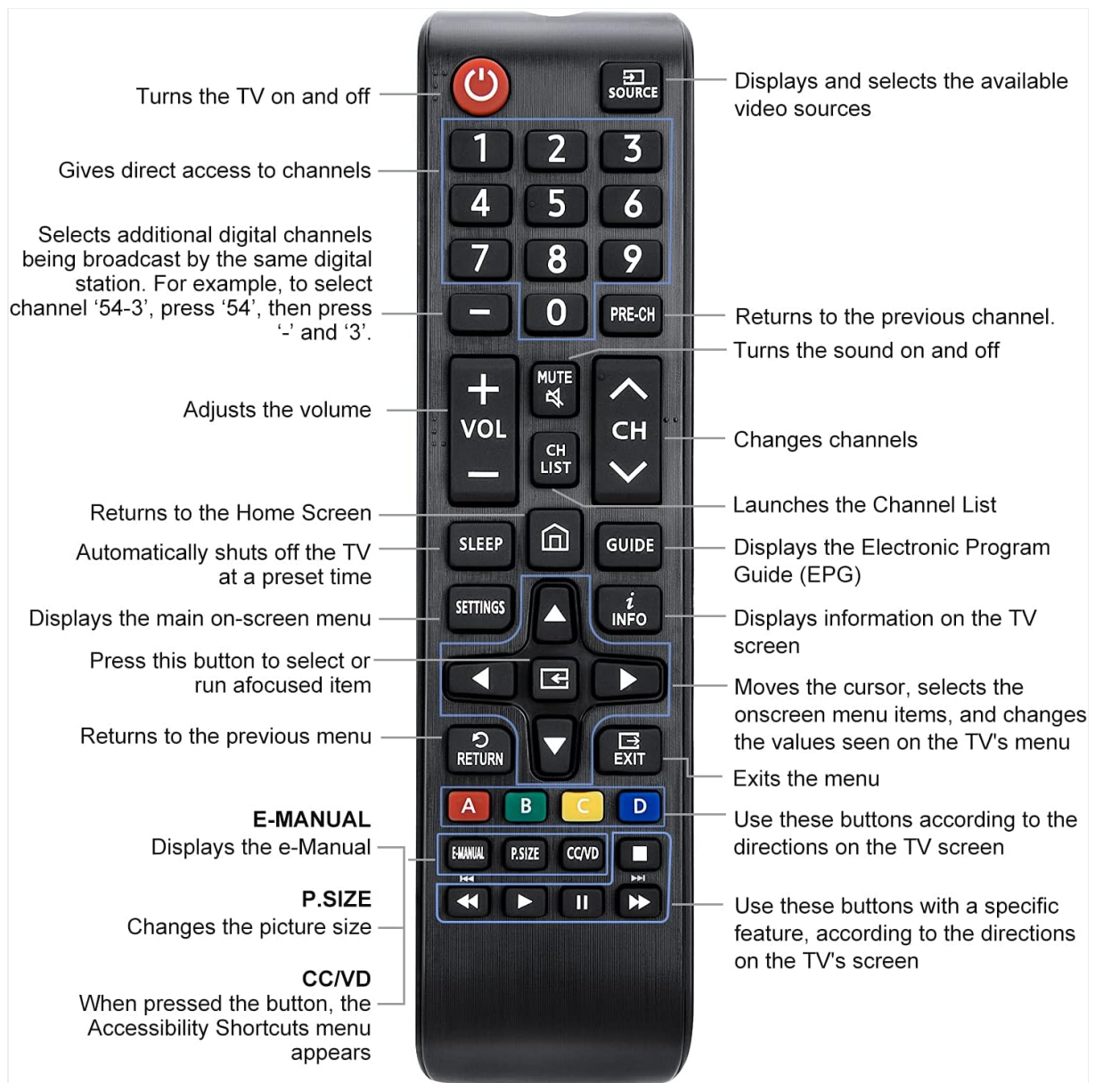
Image 3.1: Detailed layout of remote control buttons and their corresponding functions.
