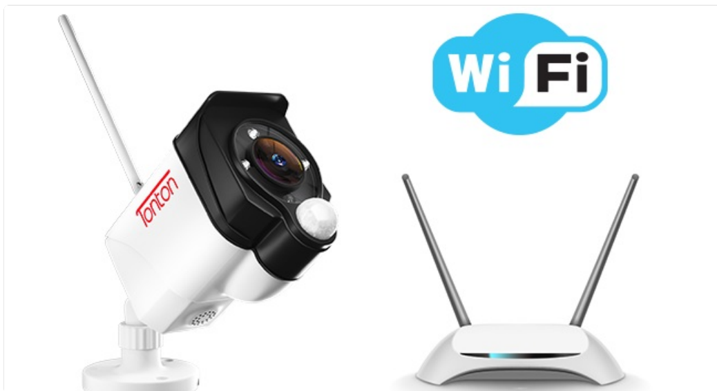
Figure 4: Wi-Fi Connection. The camera connects wirelessly to your 2.4GHz Wi-Fi network.
