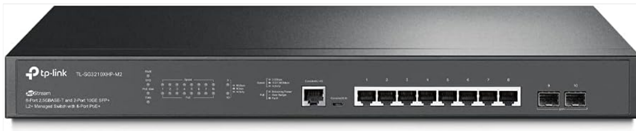
Figure 1: Front view of the TL-SG3210XHP-M2 switch, showing the TP-Link logo, model number, LED indicators, 8x 2.5Gbps PoE+ ports, and 2x 10G SFP+ slots.
