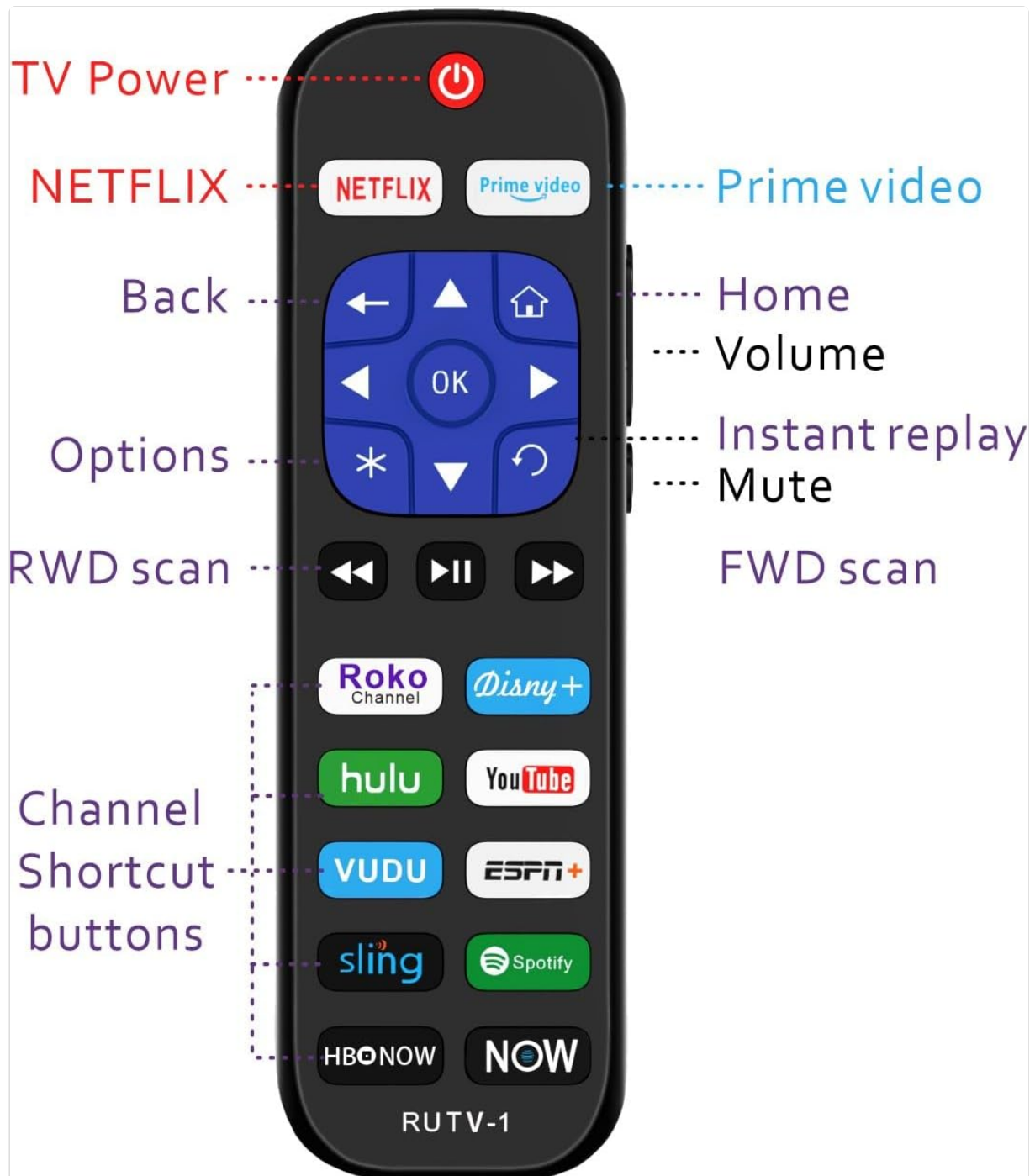
Figure 2: Labeled diagram of the Alizen Remote Control.
