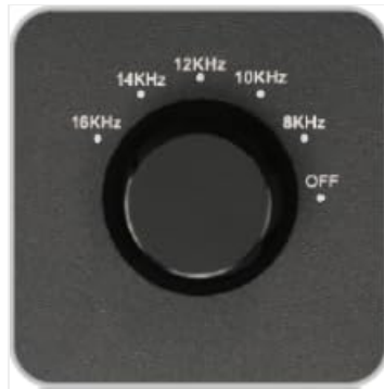
Image: Detail of the crossover frequency selection knob.
