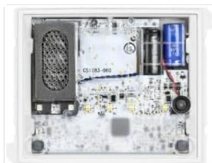
Figure 1: Internal view of the Urmec Alpha Audio External Station, showing the circuit board, speaker, microphone, and electronic components. This image provides a detailed look at the internal layout of the device.
