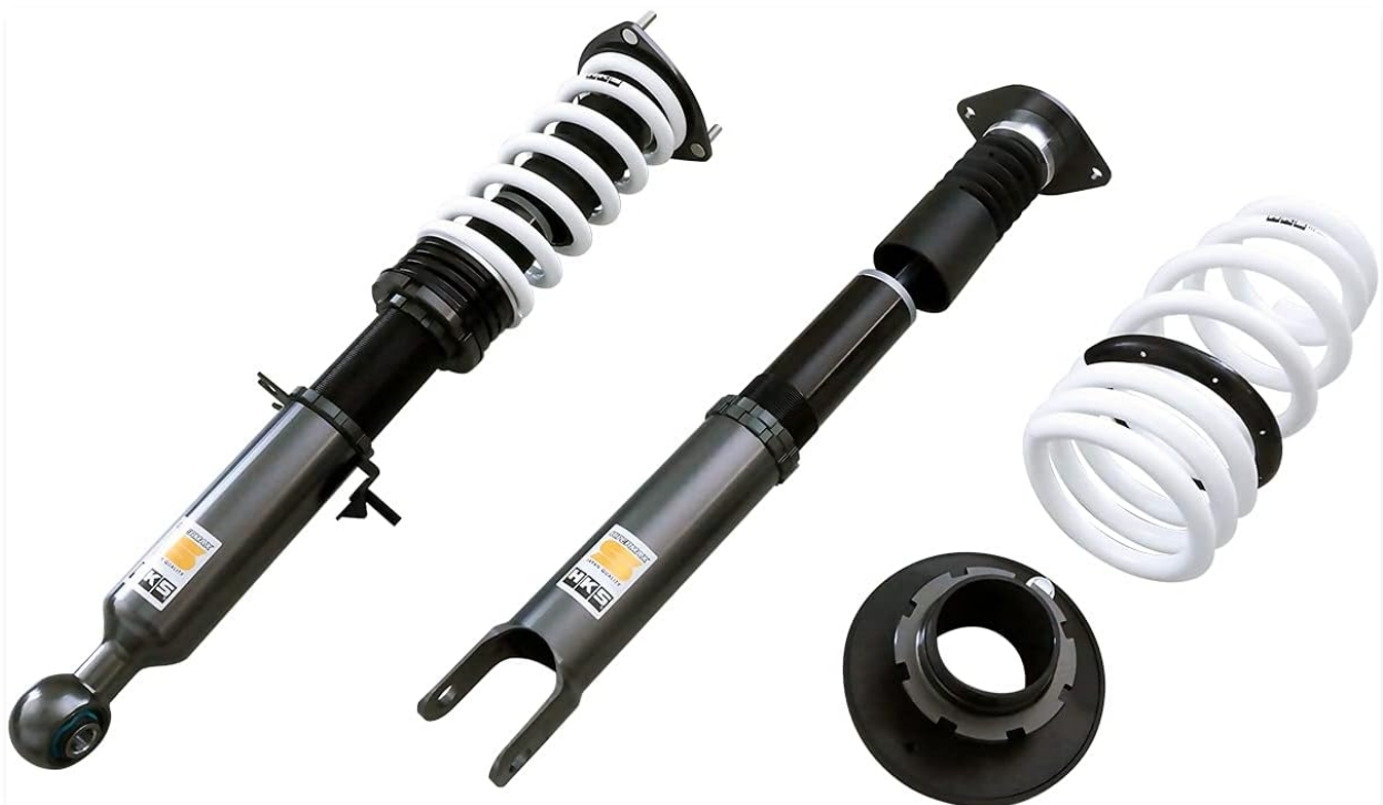
Image 1.1: Overview of HKS Hipermix S Series Coilovers components, including front and rear shock absorbers with springs, and adjustment tools.
