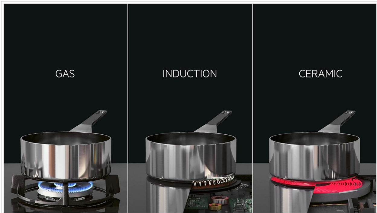
Image 3.2: Visual comparison illustrating the heating principles of gas, induction, and ceramic hobs, highlighting the direct and efficient heating of induction technology.
