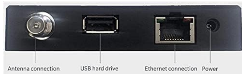
Image: Rear ports of the HDHomeRun Flex Duo, showing connections for antenna, USB hard drive, Ethernet, and power.
