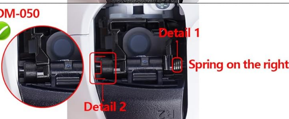
Image: Visual guide for distinguishing PS5 controller BDM models by R2 trigger components.
