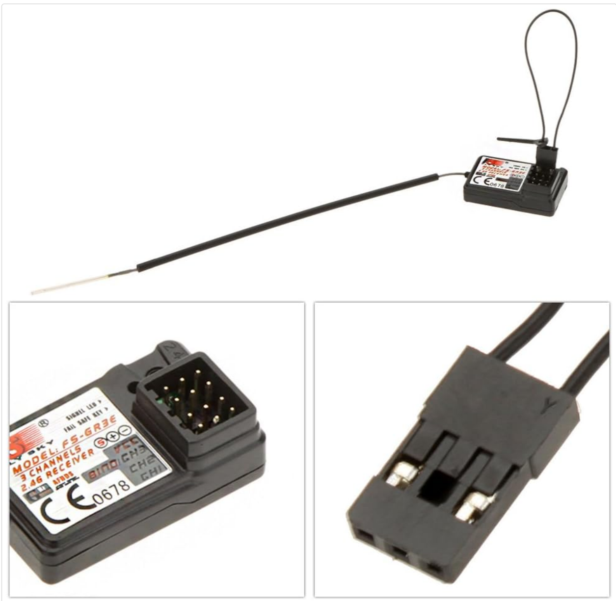
Image 1.1: The Goolsky Flysky FS-GR3E receiver, showing its compact size, antenna, and the bind plug connected to the BIND/CH3 port.
