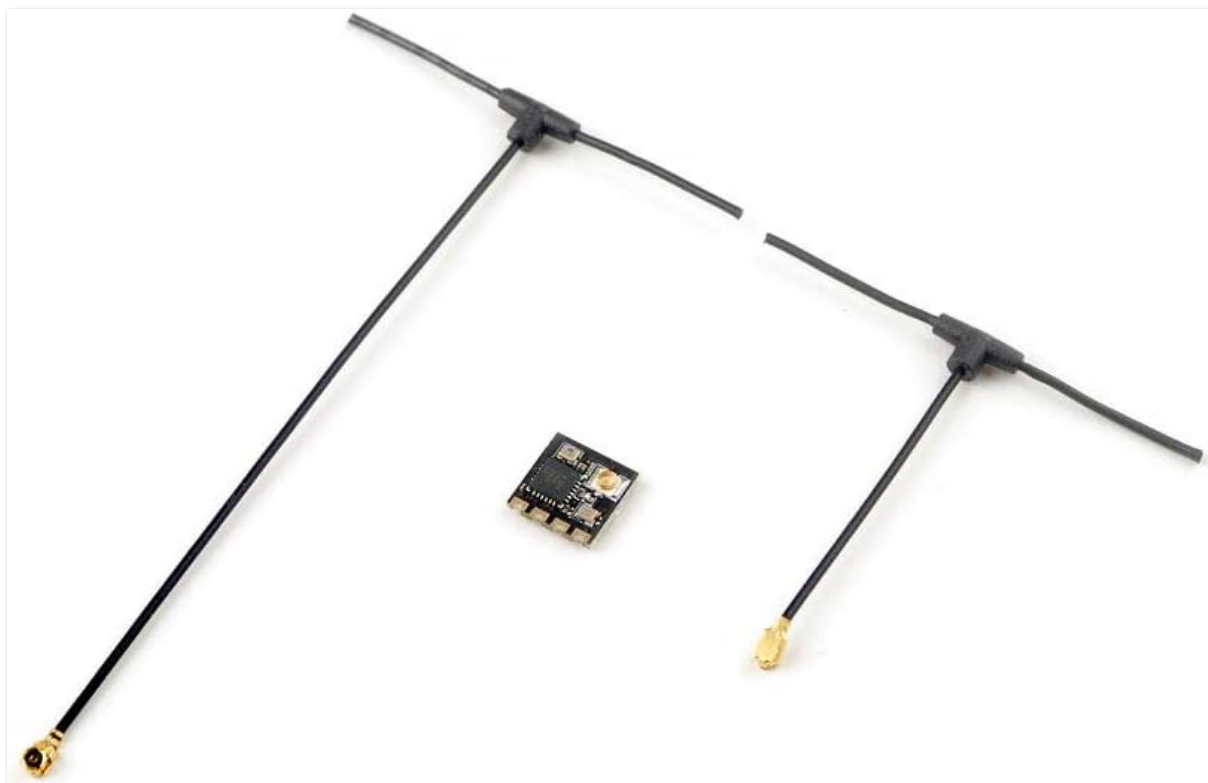
Figure 1: Happymodel ELRS EP1 RX receiver module with two dipole antennas. This image displays the compact receiver and its two attached antennas, illustrating the complete unit.
