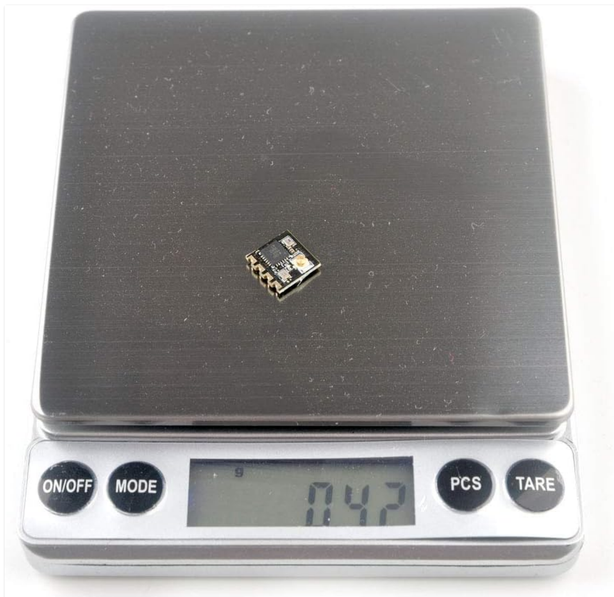
Figure 3: Happymodel ELRS EP1 RX receiver on a digital scale. This image demonstrates the ultra-light weight of the receiver, measuring 0.42 grams.
