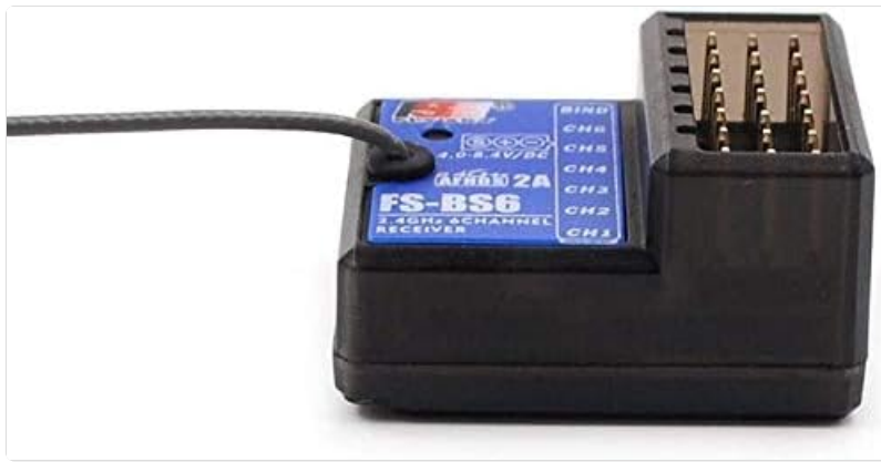
Image 3: Detailed view of the FS-BS6 receiver's channel ports (CH1-CH6) and BIND port, ready for component connections.
