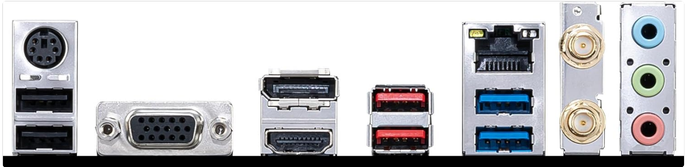
Image: A detailed view of the motherboard's rear input/output (I/O) panel, showing various ports including USB, Ethernet, DisplayPort, HDMI, and audio jacks.
