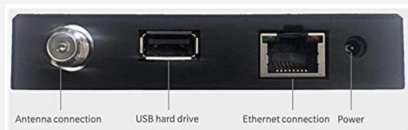
Image: Rear panel of the HDHomeRun Flex 4K, showing the antenna connection, USB hard drive port, Ethernet connection, and power input.
