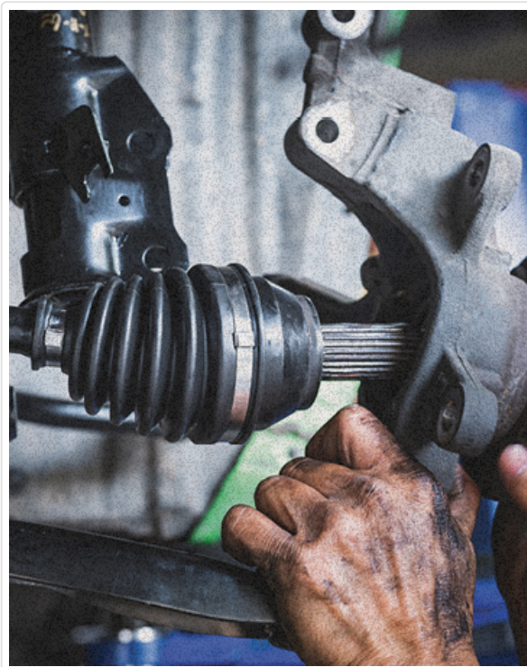
Image 5.2: A close-up view of an ATV axle, highlighting the area where the CV boot is installed.
