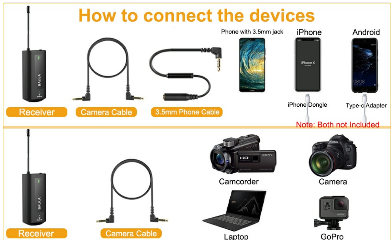
Figure 10: Connection guide for the receiver to different devices. Use a 3.5mm TRS cable for cameras/laptops and a 3.5mm TRRS cable for smartphones (iPhone/Android). Note: iPhone dongle and Type-C adapter are not included.
