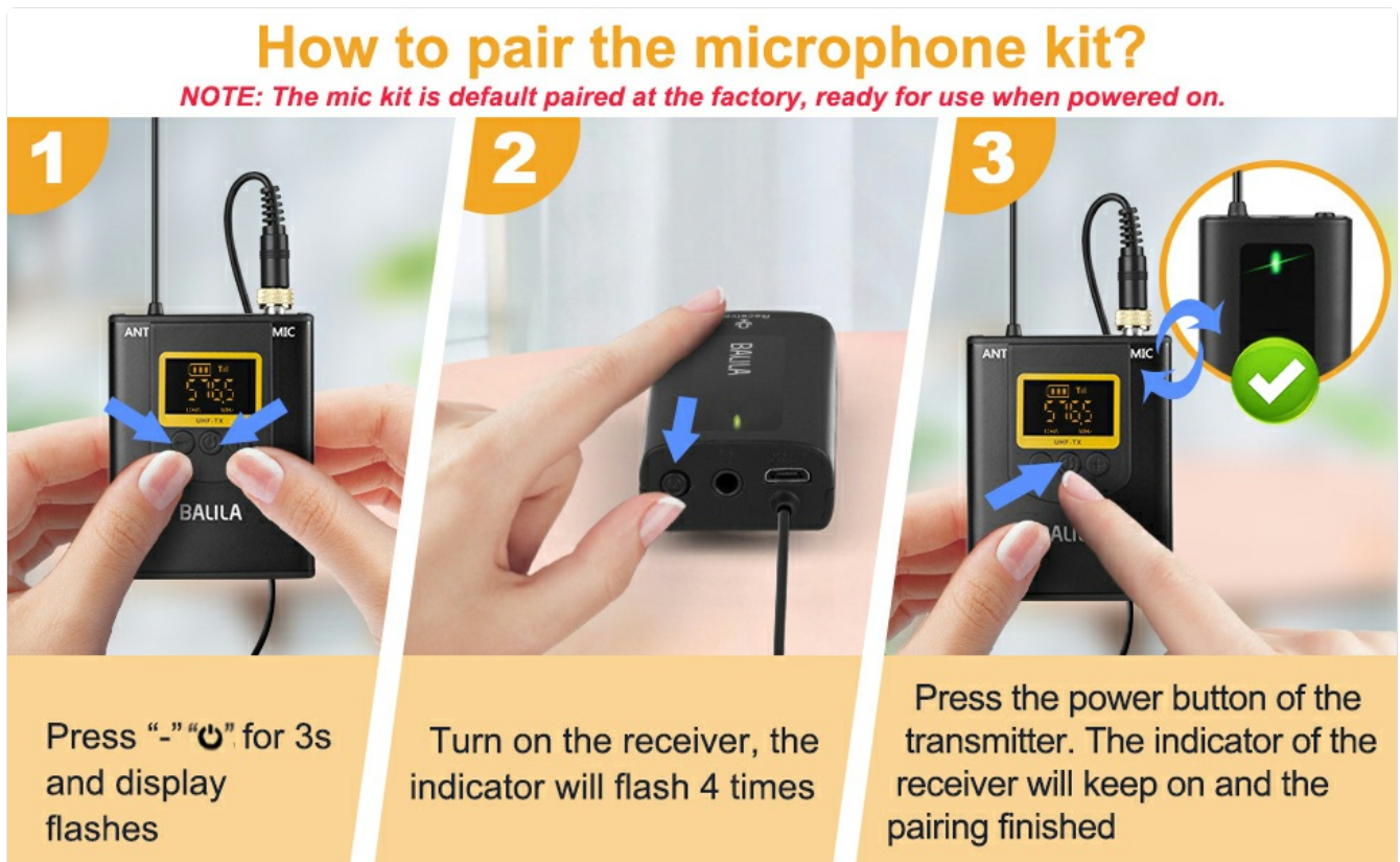
Figure 11: Step-by-step visual instructions for pairing the BALILA microphone transmitter and receiver.
