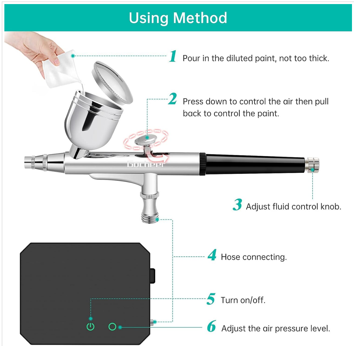
Figure 2: Step-by-step Airbrush Usage Method
