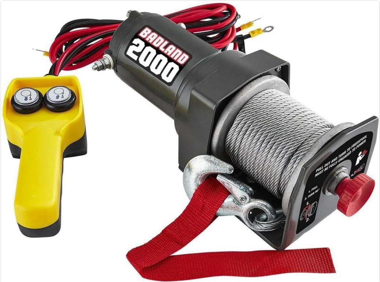
Figure 5.1: Close-up view of the winch showing the free spooling clutch mechanism. To engage, pull out and turn the red knob.
