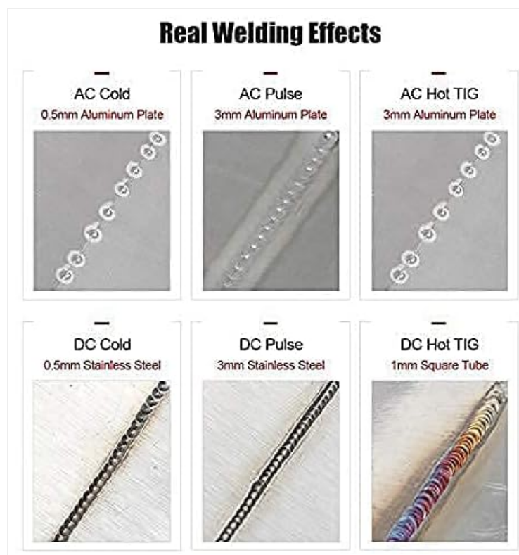
Figure 5.1: Examples of welding results using the ANDELI TIG-250PLS. This image showcases various weld types including AC Cold, AC Pulse, AC Hot TIG on aluminum, and DC Cold, DC Pulse, DC Hot TIG on stainless steel and square tube, illustrating the machine's versatility.
