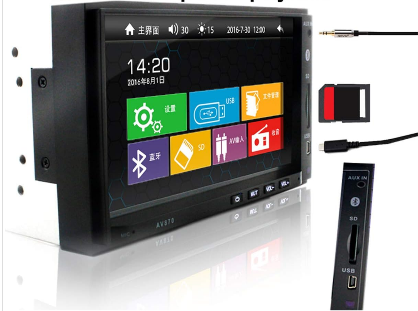
Image: The AV870 car stereo showing its USB, AUX, and SD card input options, along with compatible media devices.
