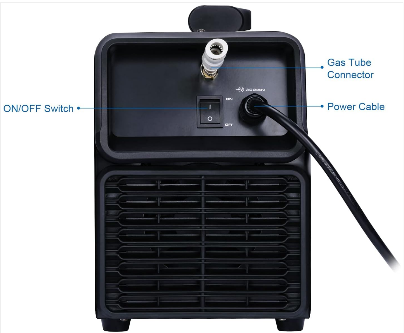
Figure 3: Rear Panel Connections
