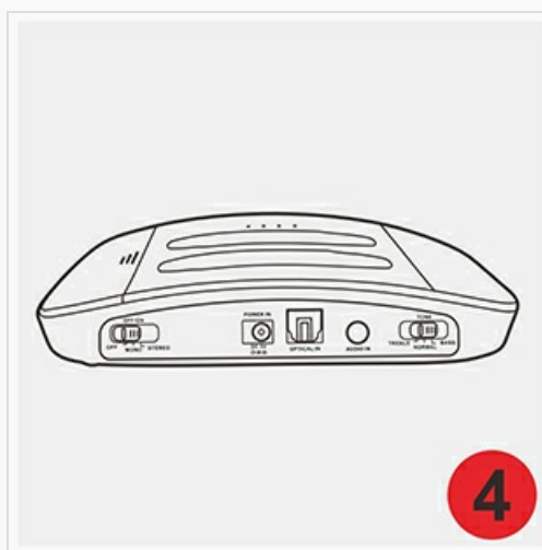
Image: Rear view of the transmitter, highlighting the input ports and audio mode switches.
