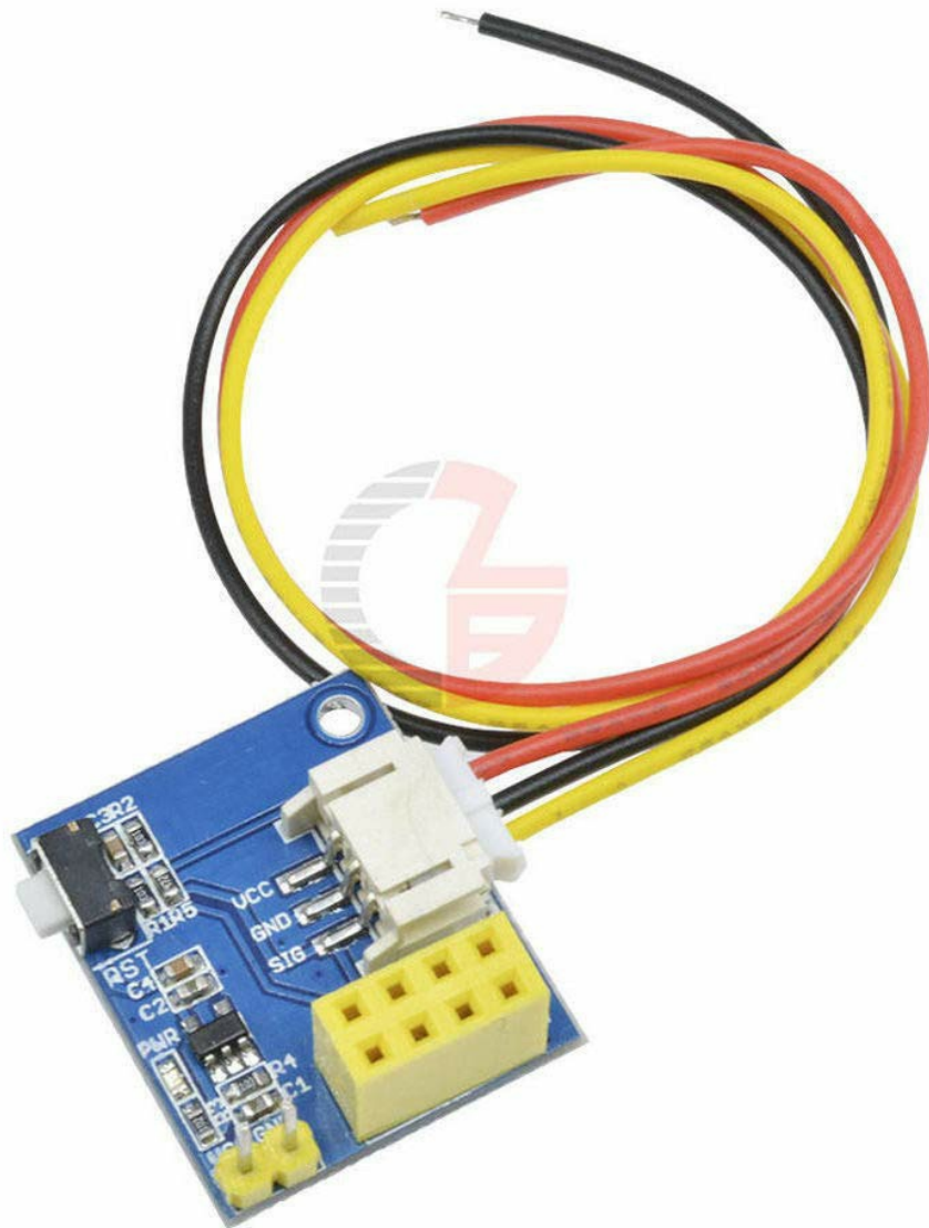
Figure 1: Top view of the ESP-01S RGB LED Controller Module with connected 3-pin wires.
