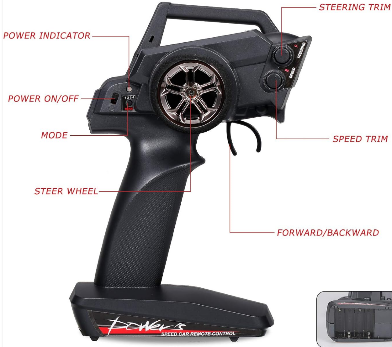
Image 4.1: Labeled diagram of the 2.4GHz remote controller, showing Power Indicator, Power ON/OFF switch, Mode button, Steer Wheel, Steering Trim, Speed Trim, and Forward/Backward trigger.
