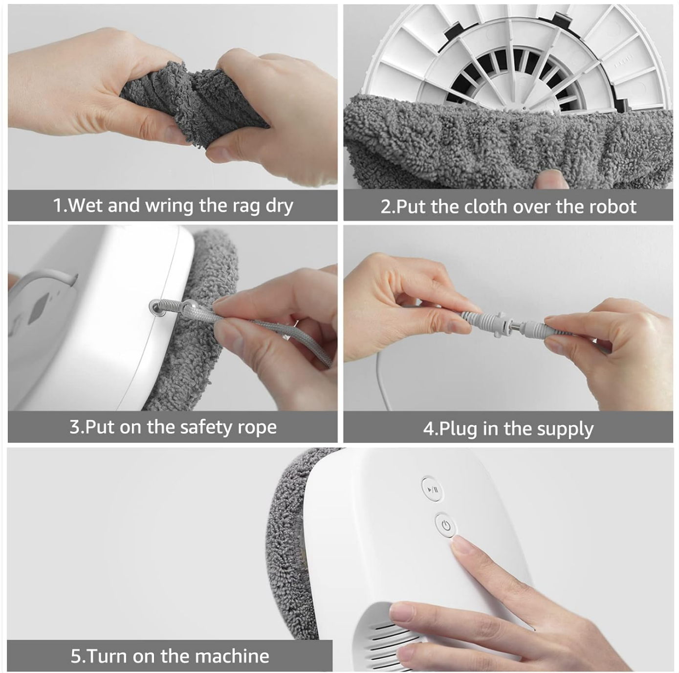
Figure 5.1: Step-by-Step Setup. This visual guide demonstrates the five essential steps for preparing the HUTT DDC55 for operation: wetting and wringing the cloth, attaching it to the robot, securing the safety rope, plugging in the power supply, and finally, turning on the machine.
