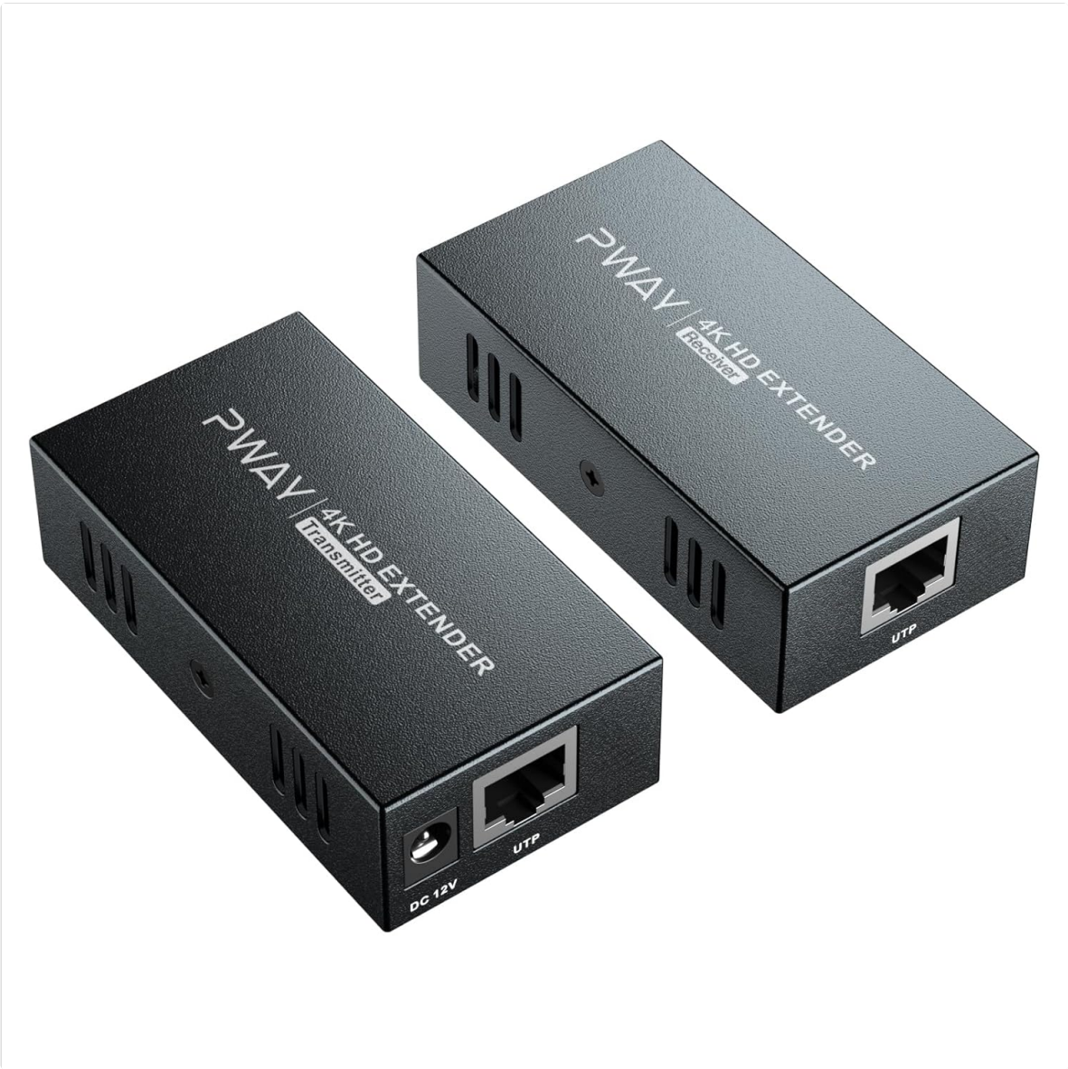
Image 3.1: The PWAYTEK 4K HDMI Extender Transmitter and Receiver units, showcasing their compact design and port labels.
