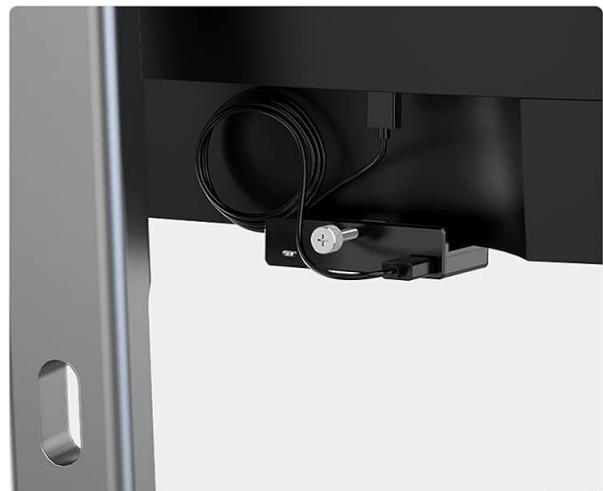
04 Step3: Connect the hub to computer USB port
