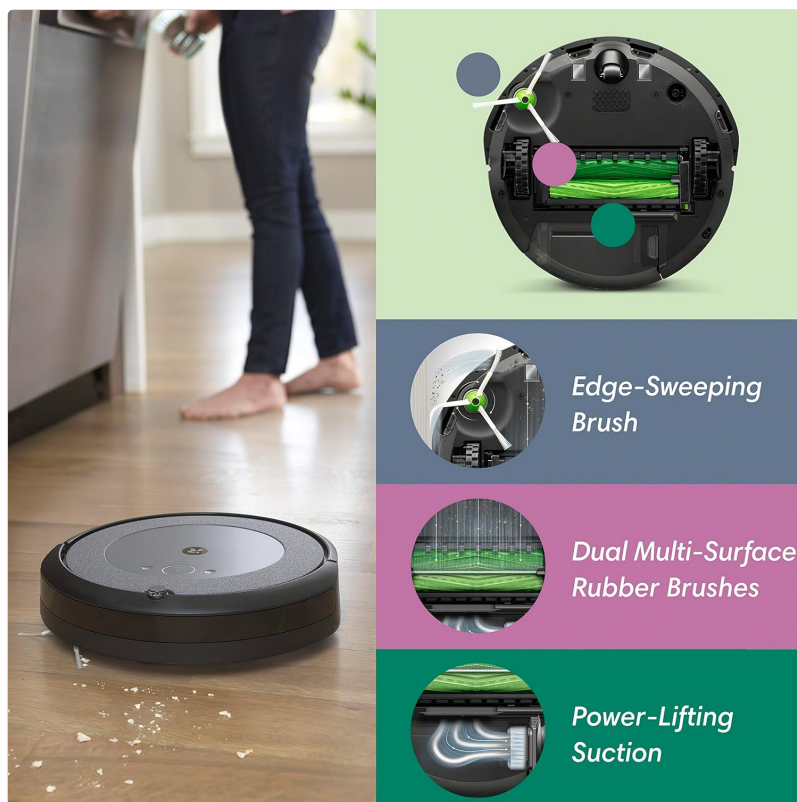
Image: A diagram showing the underside of the Roomba i4 EVO, highlighting the Edge-Sweeping Brush, Dual Multi-Surface Rubber Brushes, and Power-Lifting Suction components.
