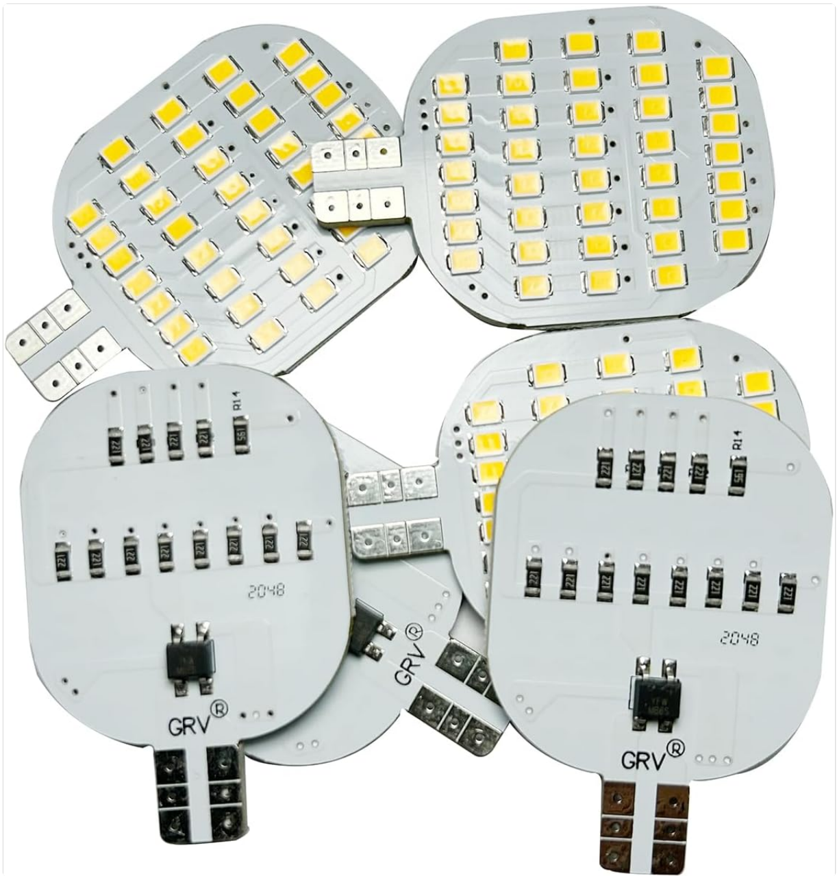
Figure 4.2: Rear view of several GRV T10 LED bulbs, showing the circuit board and contact pins.
