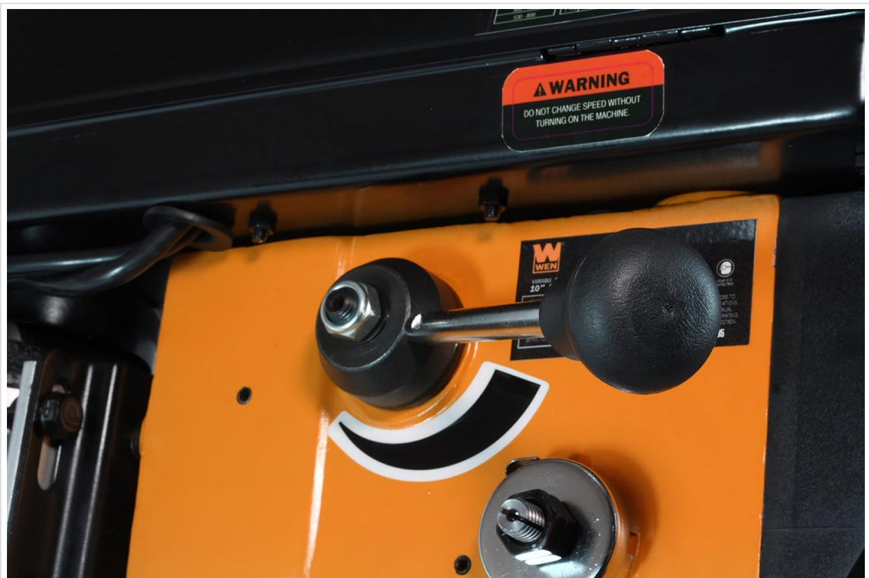
Figure 4: Variable Speed Adjustment Lever
