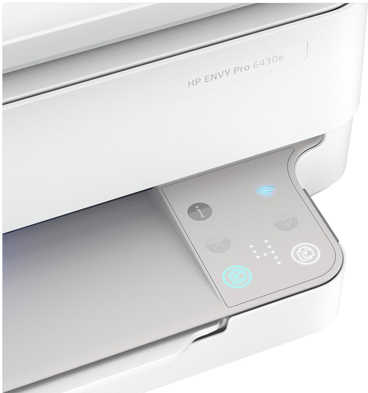
Image 1.2: Close-up of the HP Envy 6430e control panel, showing touch-sensitive buttons for Wi-Fi, information, and other functions.
