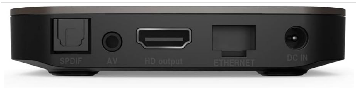
Figure 3.2: Rear panel of the TVBOX. From left to right, the ports include: SPDIF (digital audio output), AV (analog audio/video output), HD output (HDMI port for high-definition video and audio), ETHERNET (for wired network connection), and DC IN (power input).
