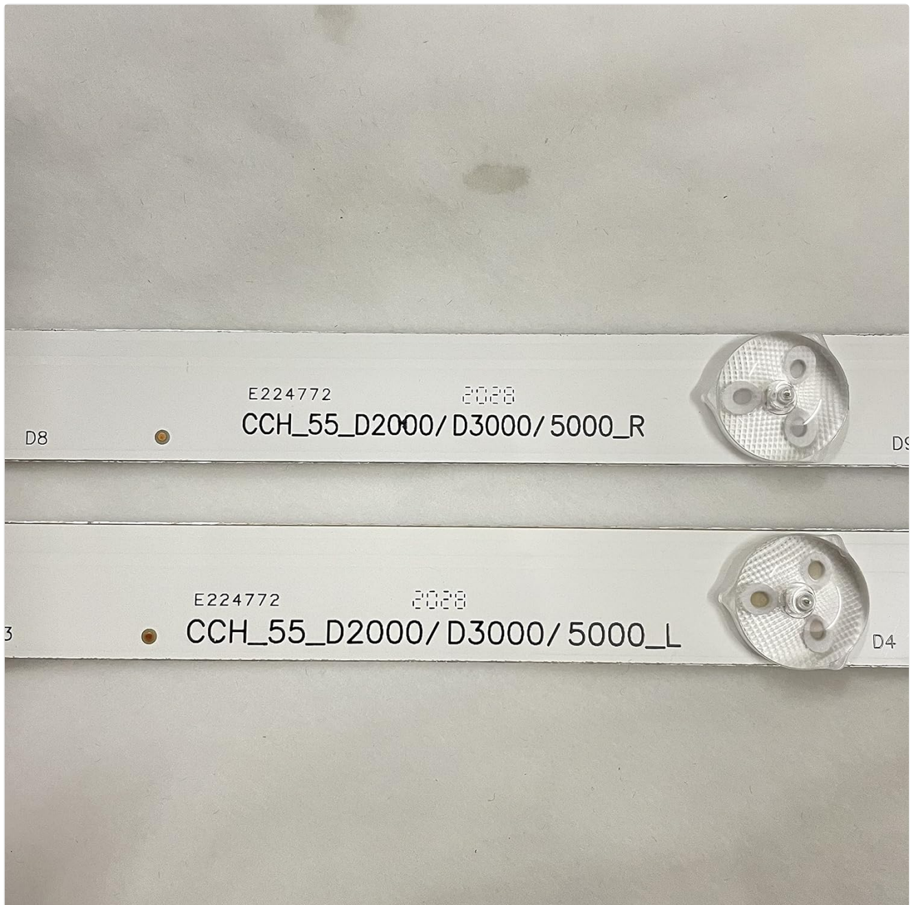
Figure 2: Detailed view of the markings on the LED backlight strips, showing "CCH_55_D2000/D3000/5000_R" and "_L". These markings are critical for verifying compatibility with your existing strips.
