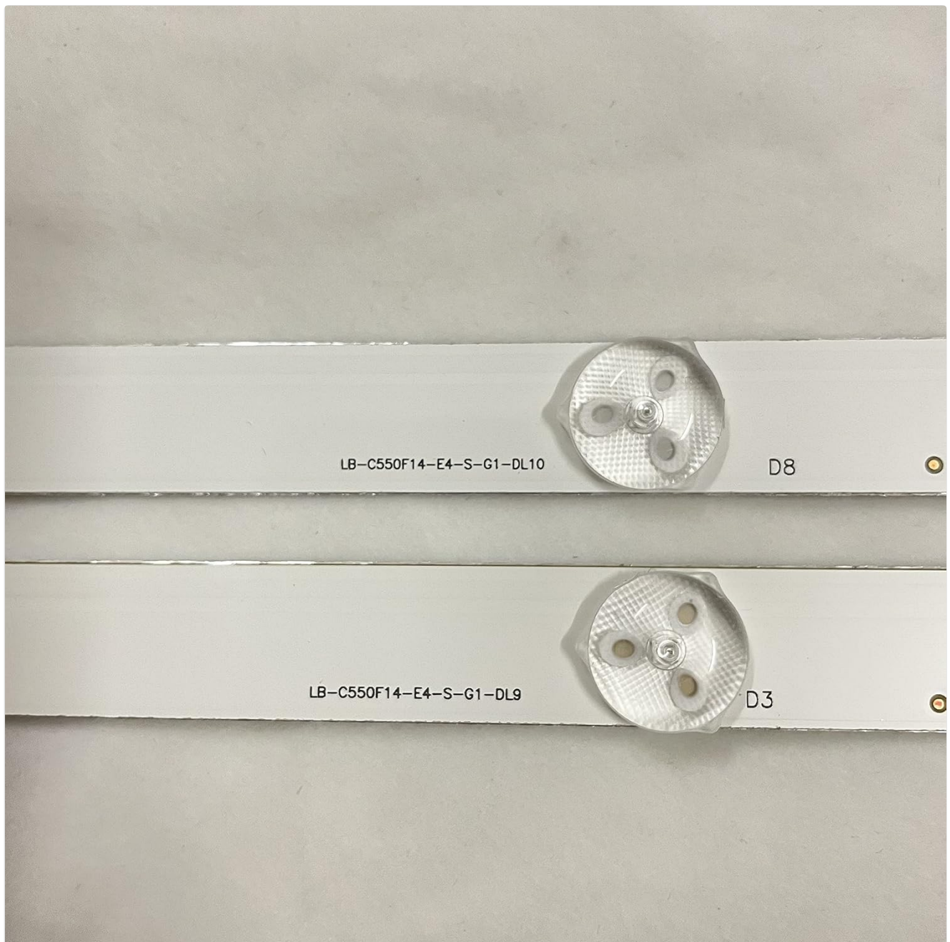
Figure 3: Another close-up showing specific model identifiers "LB-C550F14-E4-S-G1-DL10" and "-DL9" on the LED backlight strips. Match these numbers to your original strips for accurate replacement.
