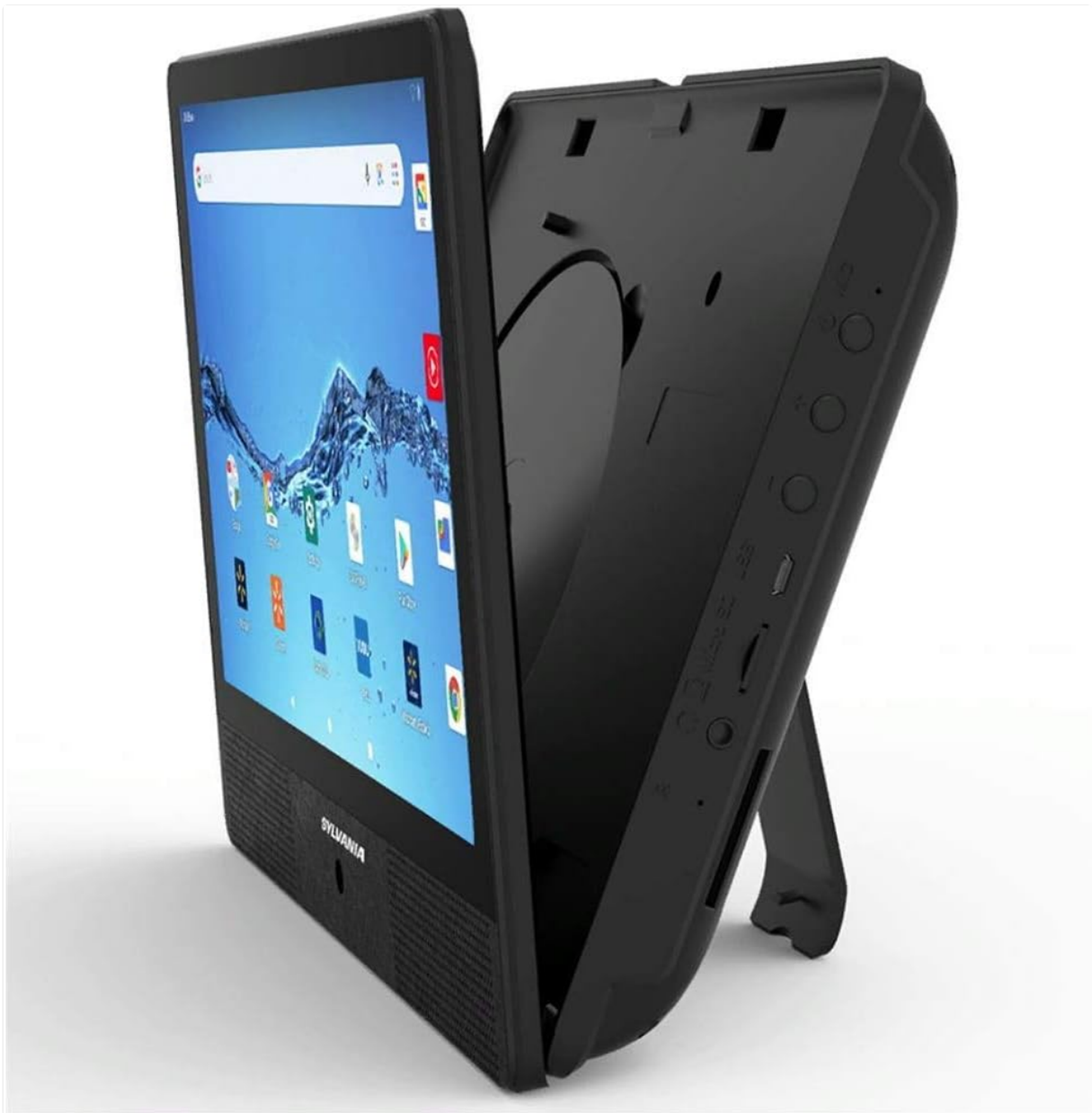
Figure 3.3: Rear angled view highlighting the integrated kickstand for hands-free viewing and various input/output ports on the side.
